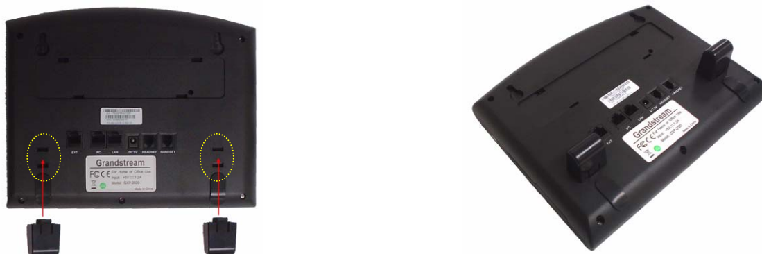
Figure 2: Attaching the Wall-Mount Spacers
